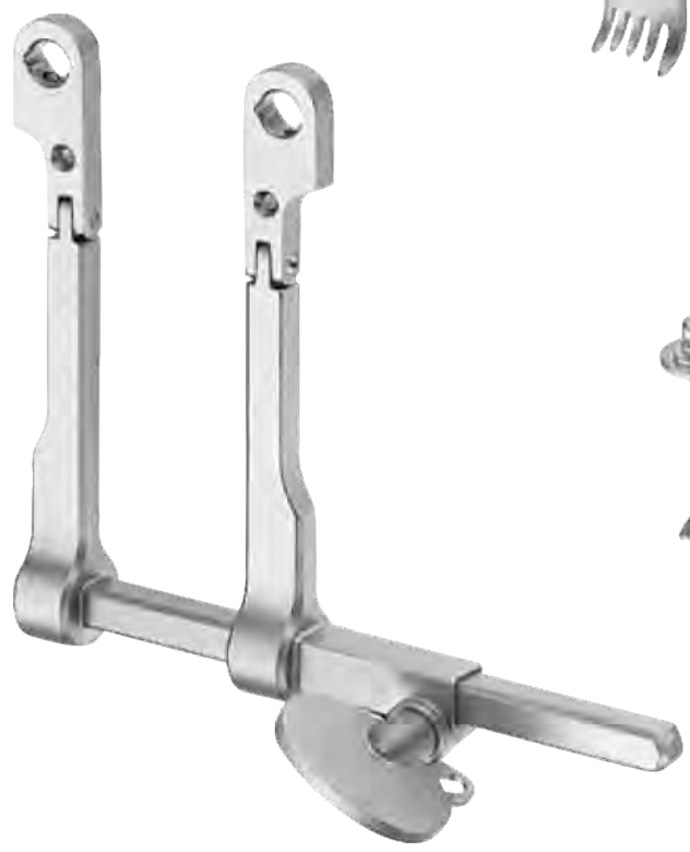
CASPAR UV-272 Caspar Cervical Spine Retractor stainless steel, complete set for transverse retraction, 65 mm spread, adjustable, with 5 medial and 5 lateral stainless steel, blades 40, 45, 50, 55, 60 mm
